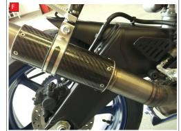
A) Remove lower fairing bolt to aid access to OE silencer clamp
